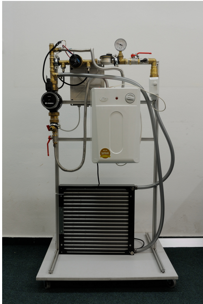
Figure 4.1: Physical hydronic network model.
